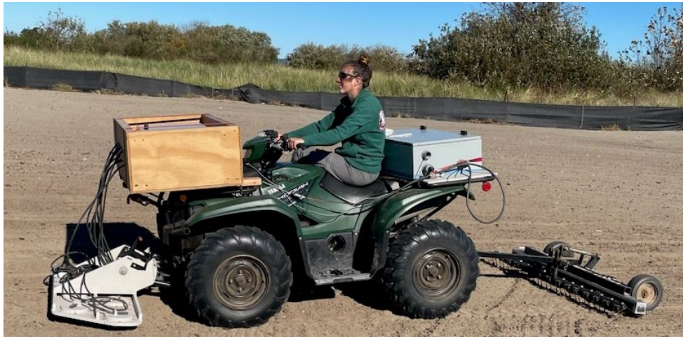
Figure 4. A photo displaying PIT tag recovery equipment installed on an ATV and in-use at the East Sand Island Caspian Tern colony. Photo by Noah Strong 2023.
